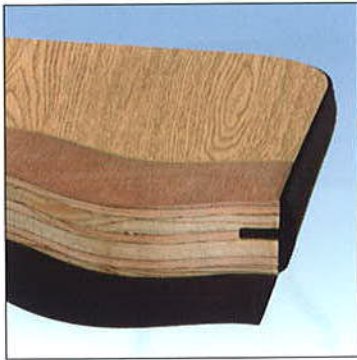
Solid 3/4" thick plywood is surfaced with high pressure plastic laminate, sealed with a backing sheet and edged with vinyl T-molding.
