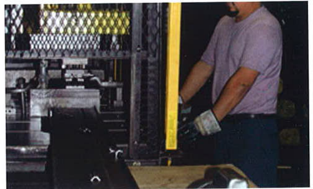
A wide variety of simple and complex formed steel parts are produced in a continuous process. Coil steel is de-burred and blanked to size and shape. The steel blank is then formed to final shape with progressive, precision forming dies to produce finished parts that are the exactly the same with each stroke of the automatic press.
