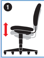
1. Pneumatic Seat-Height Adjustment Regulates height of chair relative to floor.
