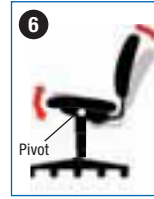
6. Tilt Pivot point located directly above center of chair base.
