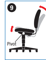
9. Dual-Action Synchro Tilt Back reclines at a 2-to-1 ratio to seat angle. Allows user to recline while keeping seat cushion relatively level to floor.
