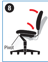
8. Knee Tilt Pivot point located near front edge of chair. Allows user to keep feet flat on floor while chair reclines.
