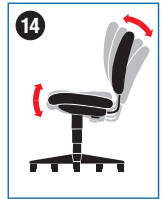
14. Asynchronous Control Three levers modify: • Angle of back relative to seat • Tilt (free float or infinite locking within a fixed range) • Forward tilt
