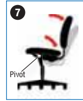
7. Mid-Range Knee Tilt Pivot point located slightly ahead of center of chair base. Allows user to recline at a slightly more relaxed angle than conventional tilt.
